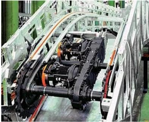
Diagram 6.27 View of an Internal Drive Machine used in escalator (Left) Components within an Internal Drive Machine(Right)
