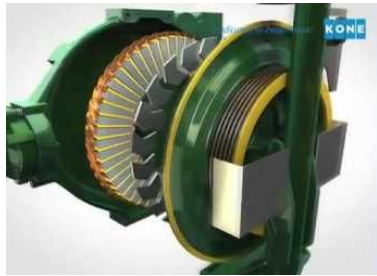
Diagram 6.12 Sheave as a gear for traction elevator
